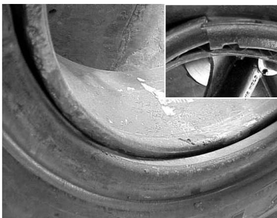
*Inner wheel with tire mounted. Inset: Close-up of split rim against mounted tire.*
