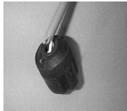
Flexible cords must be connected to devices and fittings so that strain relief is provided, which will prevent pull from being directly transmitted to joints or terminal screw.
