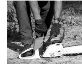
Proper way to start a chainsaw.
