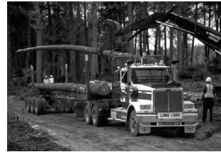
Only the machine operator and essential personnel can be in the loading and unloading work area during this operation.
