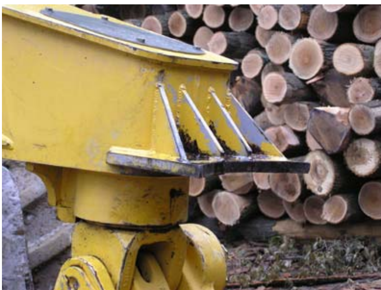
Fig. 1: Dick Cooney's "tree pusher" appliance, for improving a skidder operator's control in bringing down danger trees, consists of curved metal plate and triangular gussets welded to the back end of the grapple arch.
